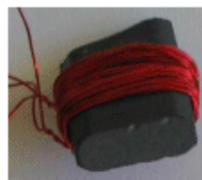
The fly-back transformer 30turns & 30 turns on any ferrite core
